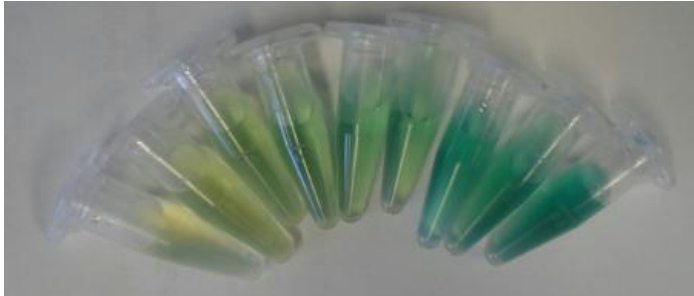
Figure 5.6 Aqueous solutions containing 0 – 80 μM NH 3 after addition of indophenol color reagents and 1 hour of color development.
