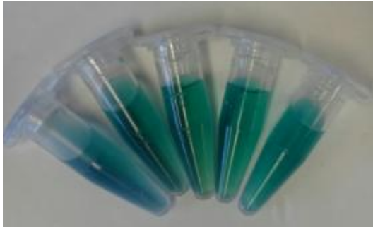
Figure 5.9 Solutions of 50 \mu\text{M} \text{NH}_3 after 1-hr color development. Preparation of \text{NH}_3 solutions from left to right: \text{NH}_3 in 20 mM Hepes, 10 mM Hepes, 5 mM Hepes, 2.5 mM Hepes, 1 mM Hepes.
