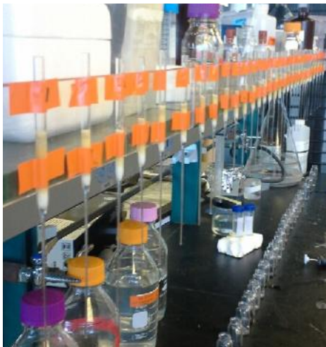
Figure 5.10 Pipet columns containing Dowex anion exchange resin used to separate \text{NH}_3 from interfering substances in the nitrogenase activity assay matrix prior to reacting with indophenol reagents.
