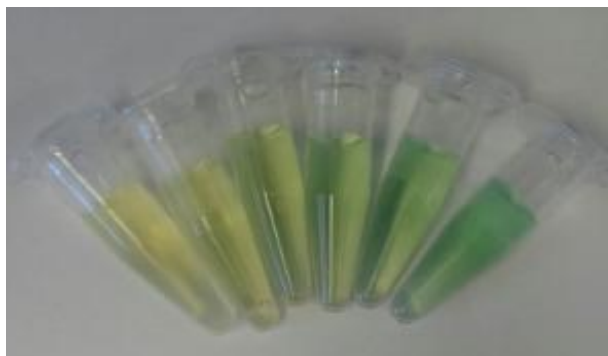
Figure 5.11 Aqueous solutions containing 0 – 80 \mu\text{M} NH 3 after elution from the Dowex pipet columns, addition of indophenol color reagents, and 1-hr color development.
