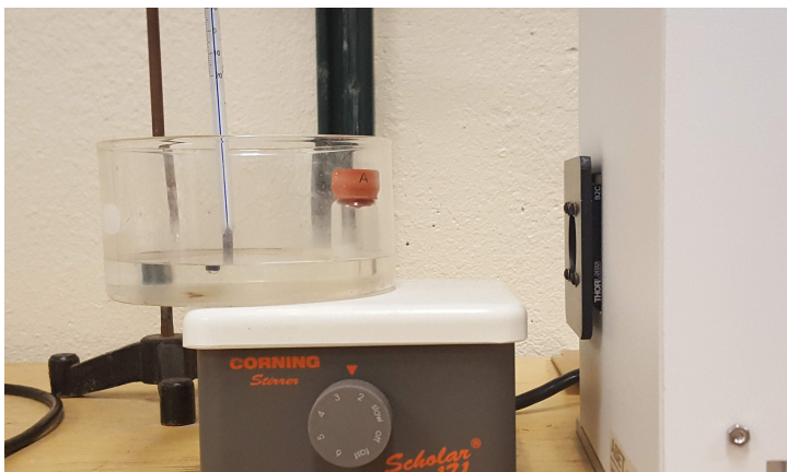
Figure 3.20 Photoreduction assay set-up with Xe arc lamp.
