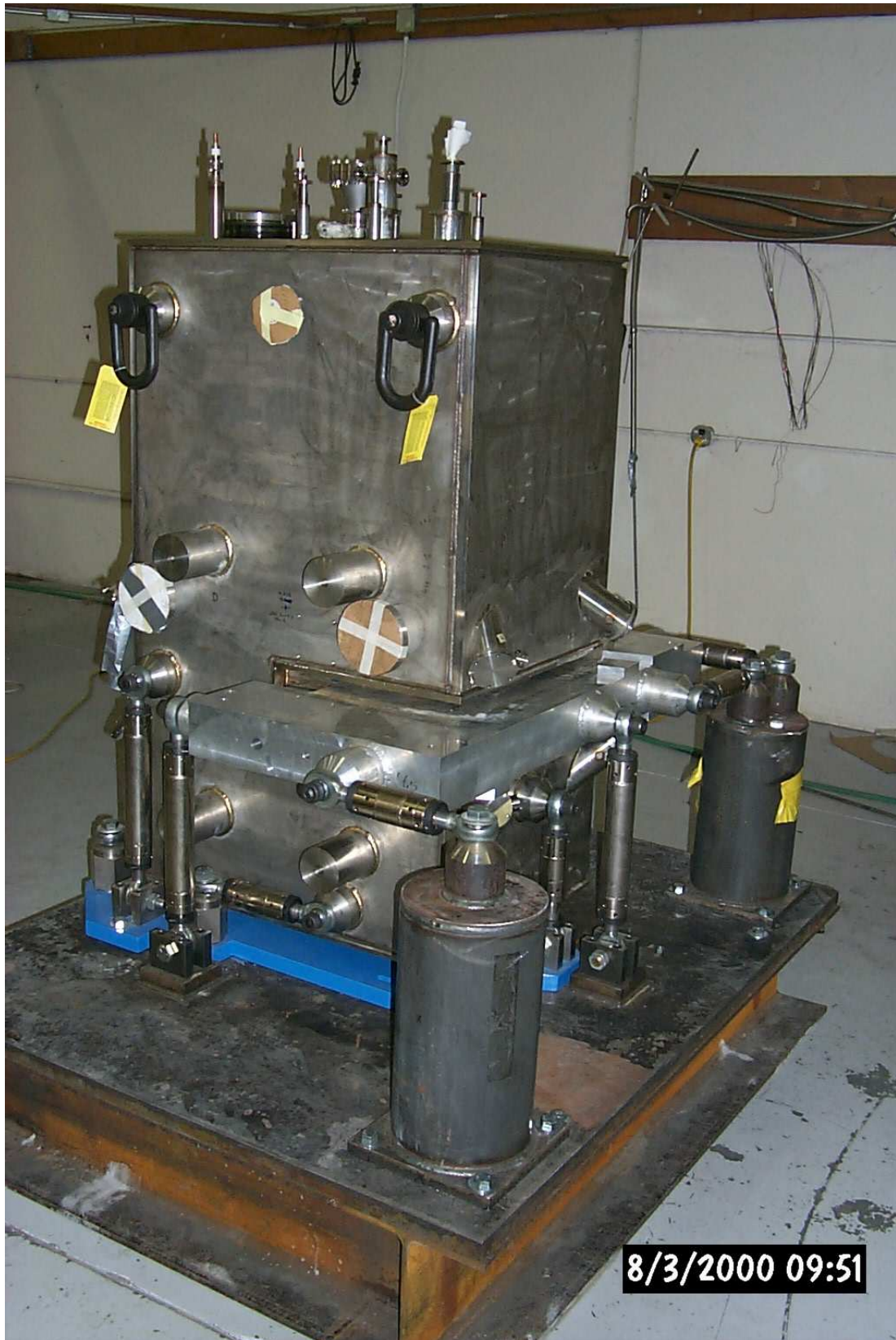
Fig. 12. First Superbend magnet installed on the test stand.
