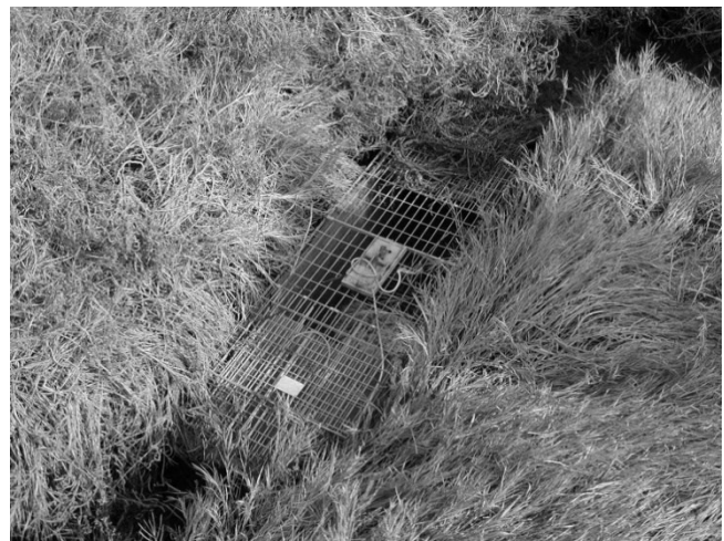
Figure 2. A Tomahawk® live trap (107 × 38 × 41 cm) modified by replacing the treadle mechanism with a tripwire attached to an externally-mounted spring-snap rat trap. Placed at low tide within channels, they passively caught California Ridgway's rails as they moved and foraged through the marsh.
