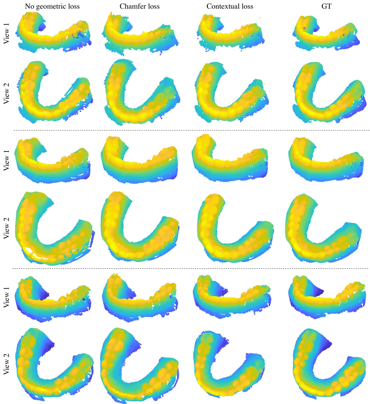
Figure 6.7: Novel view synthesis with no geometric loss, with chamfer loss and with contextual loss. Without geometric loss, the reconstructed 3D shapes suffers misalignment issues and different teeth has worse local geometric structures. Adding chamfer loss alleviate the misalignment issue, but local structures (especially for teeth near the boundary) can still improve. Contextual loss solves the misalignment issue and reconstructs the 3D dental cast with both good global and local geometric details.
