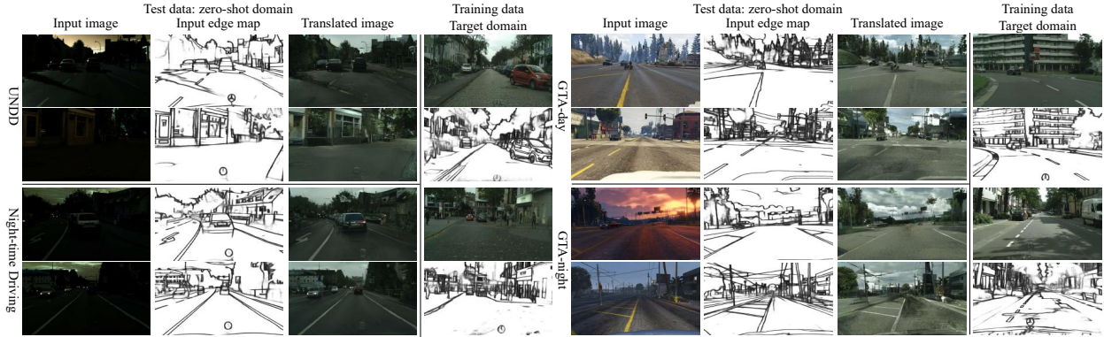
Figure 5.8: Zero-shot domain translation results. We aim to translate zero-shot images ( Left ) to the training data domain ( Right ). Specifically, we evaluate the proposed zero-shot domain translation performance on three new datasets: UNDD [209], Night-Time Driving [60] and GTA [249]. The novel domains of night-time and simulated images can be translated to the target domain of daytime and real-world images by leveraging the synthetic edge map domain as a bridge. The target domain is CityScapes dataset [56]. We extract corresponding edge maps and train an image-to-image translation model [137] to translate edge maps to the corresponding RGB images. 1st, 3rd, 5th, 7th rows of column 1 depict some sample training RGB images and 2nd, 4th, 6th, 8th rows of column 1 depict the corresponding edge maps respectively.
