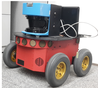
Fig. 18 The P3AT robot used to test the HCMDP planner in the real world.
