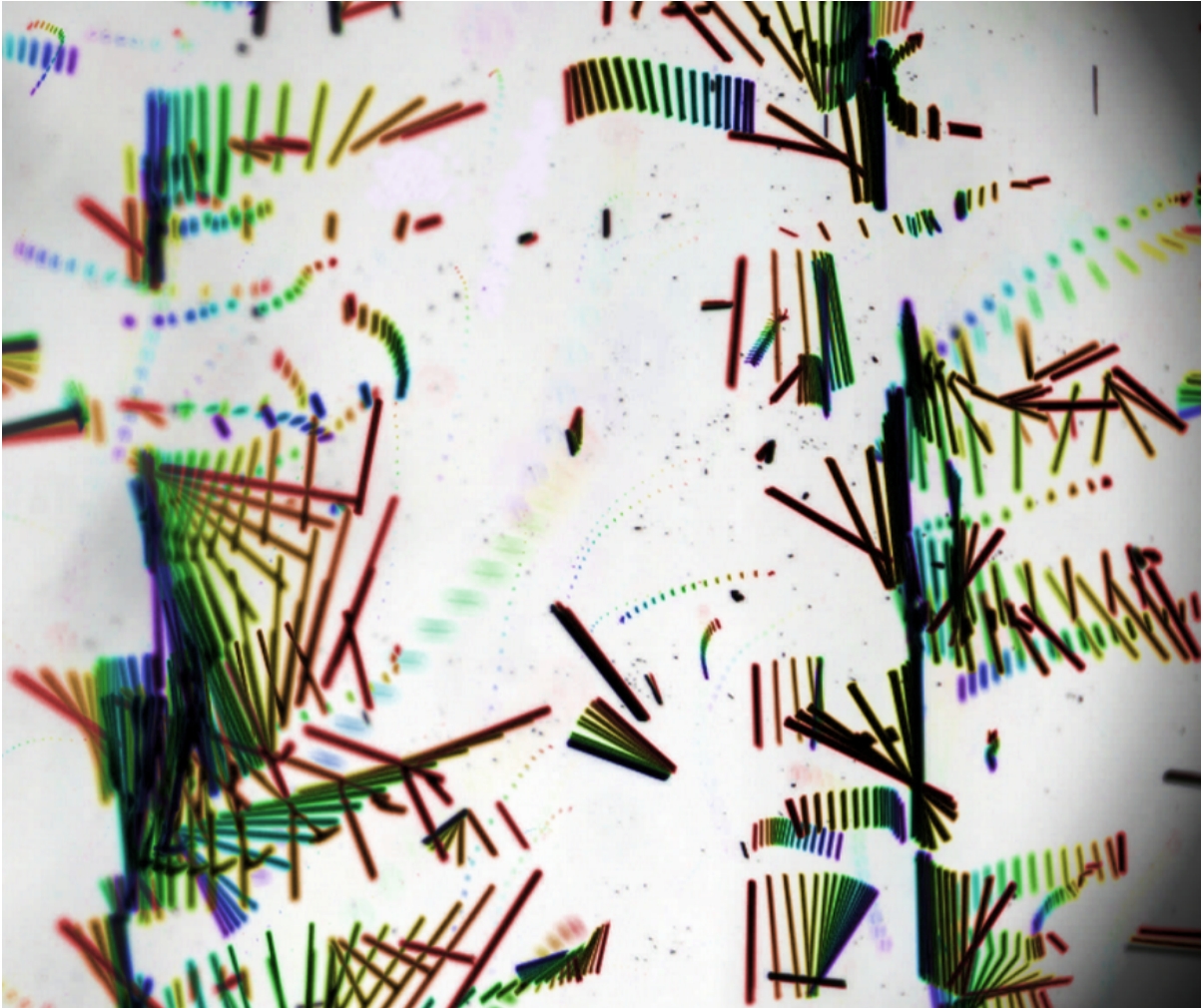
Figure 3.15: Full experimental rod trajectory image used in Figure 3.14, illustrating the positions of the low-pressure nodes.
