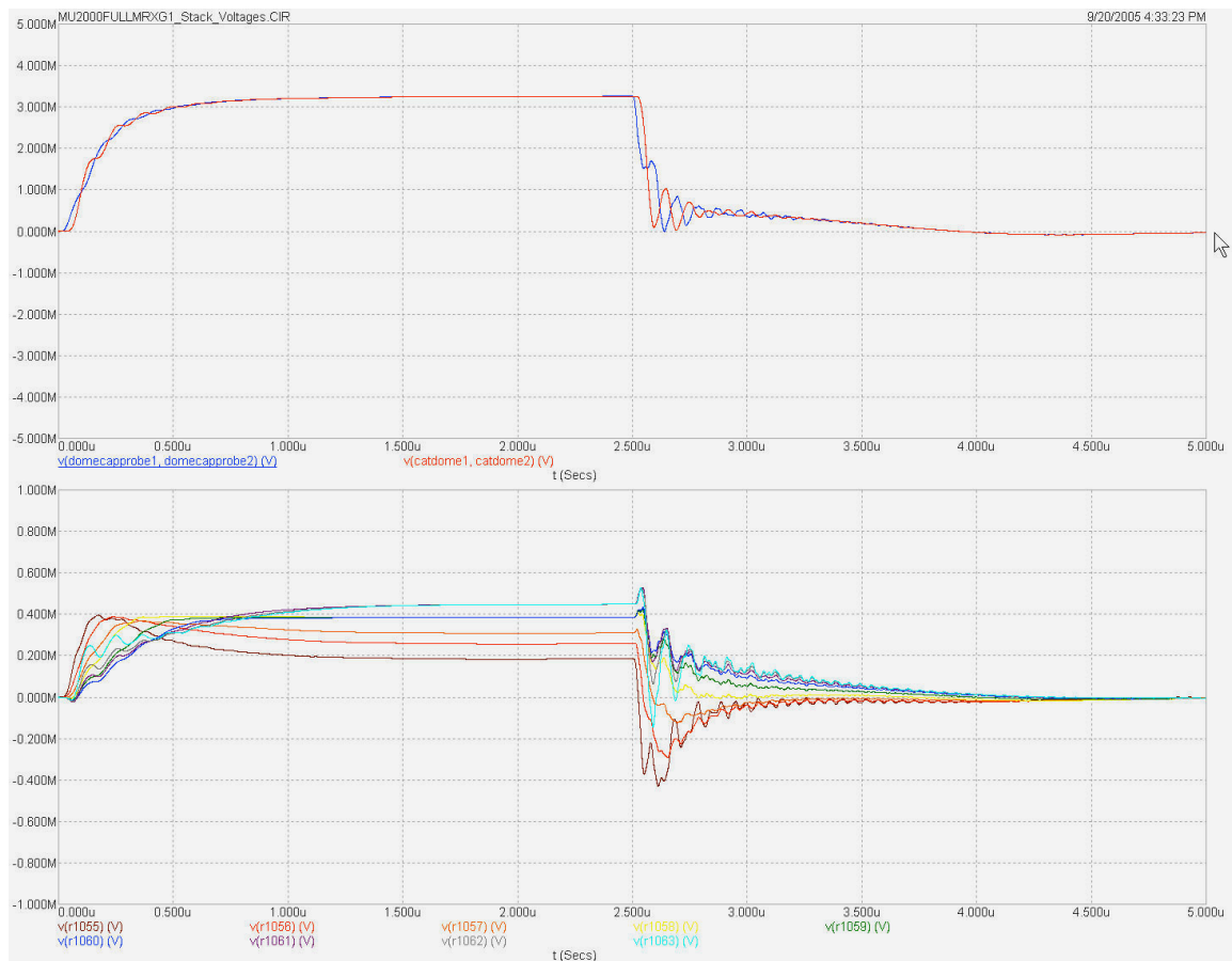
Figure 3.25 Optimum crowbar parameters: L = 2.5 \mu\text{H} , R = 45 \text{ Ohms} . Source dome (red) and Marx dome (blue) voltages in the top Figure. The nine column section voltages are shown in the bottom figure, with the lowest (brown) curve the bottom section, etc.
