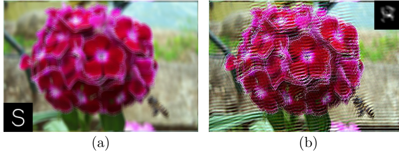
Figure 5.1: Blind deconvolution example from [6]. (a) Blurry image and the latent PSF. (b) An output deconvolved by an incorrectly estimated PSF, where we can see strong ringing artifacts.
