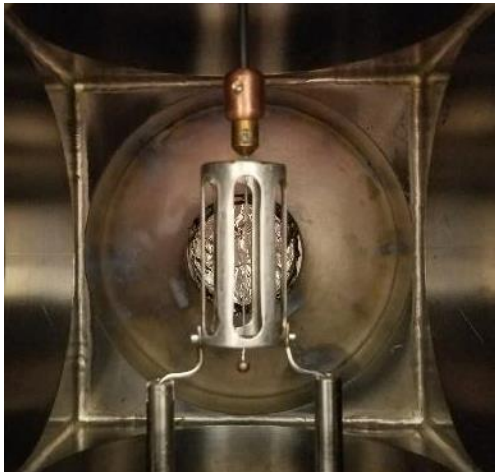
Figure 1: Schematic, top, and photo, bottom left, of the glow discharge setup in a stainless steel cube (15.2 cm edge length) with palladium wire cathode (0.5 mm diameter) in a stainless steel cage anode (2.5 cm diameter). Photo of light emission from a deuterium plasma, bottom right.
