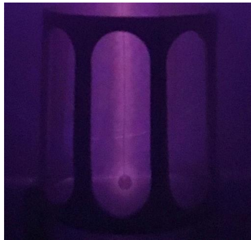
Figure 1: Schematic, top, and photo, bottom left, of the glow discharge setup in a stainless steel cube (15.2 cm edge length) with palladium wire cathode (0.5 mm diameter) in a stainless steel cage anode (2.5 cm diameter). Photo of light emission from a deuterium plasma, bottom right.
