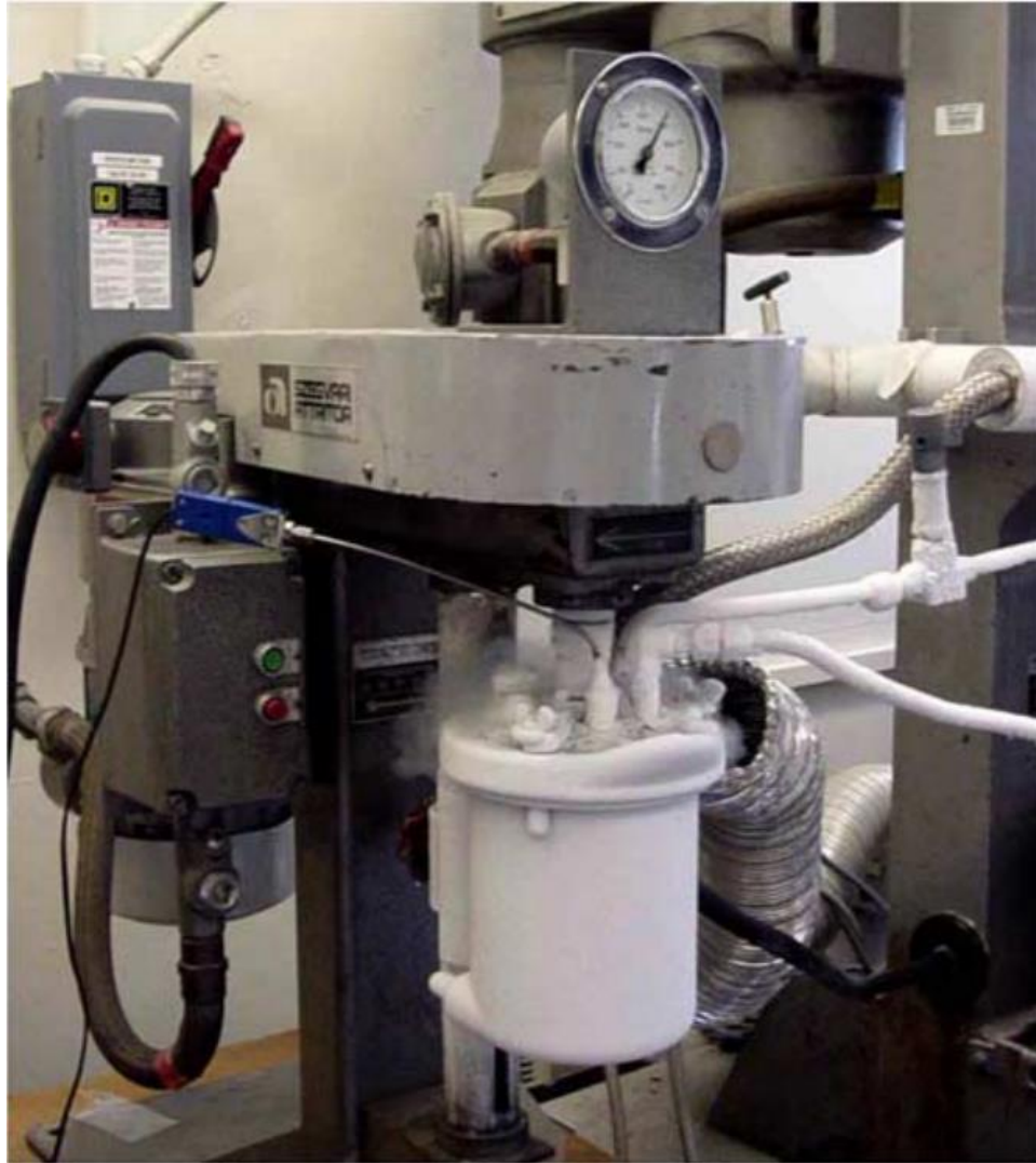
Figure 3.3: Modified attrition mill to accommodate the use of liquid nitrogen with the milling of metallic powders [49].
