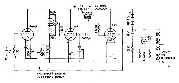
NOTE: "C" IS USED FOR INTEGRATING ELECTROMETER
