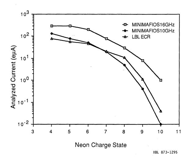
Fig. 3 Comparison of the extracted neon ion currents in e $\mu$ A for MINIMAFIOS-16GHz, MINIMAFIOS-10GHz, and the LBL ECR.
