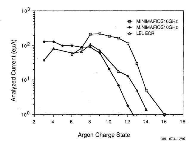
Fig. 4. Comparison of the extracted argon ion currents in e $\mu A$  for MINIMAFIOS-16GHz, MINIMAFIOS-10GHz, and the LBL ECR.
