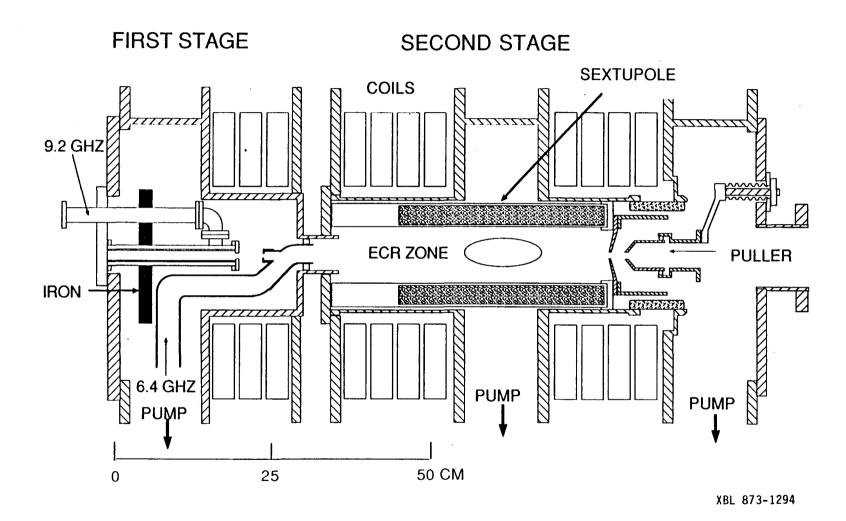
Fig. 1. Elevation view of the LBL ECR in its present configuration. The open sextupole structure allows radial pumping in the second stage.
