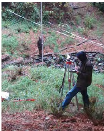
Figure 6. Surveying cross sections in the 'gabion reach,' October 23, 2010.
