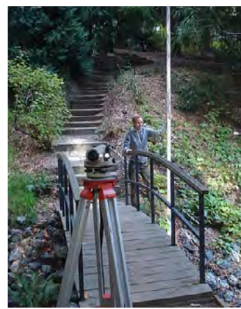
Figure 8. Surveying cross sections in the 'downstream reach,' November 5, 2010.
