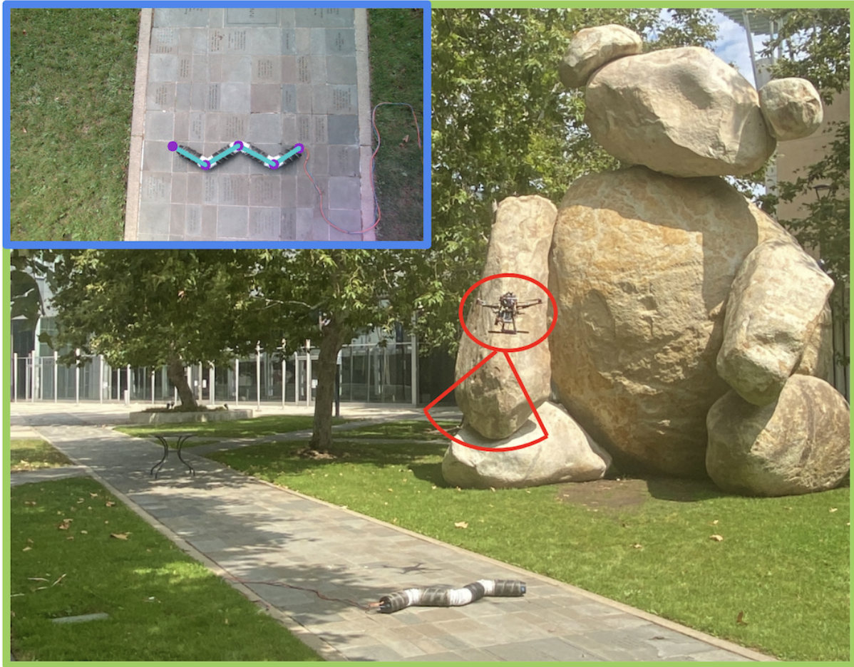
Figure 3.8. A snake-like robot, Arcsnake [105], is tracked on camera in the outdoor environment by a hovering drone.
