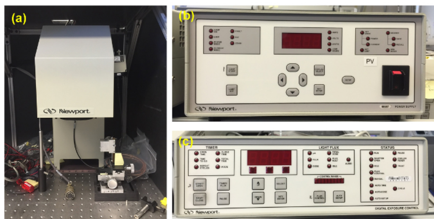
Figure 7: Standard photovoltaic measurement system. (a) Solar simulator; (b) Solar simulator controller; (c) Solar simulator flux controller. Please click here to view a larger version of this figure.
