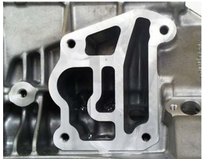
Fig. 10 Workpiece resulting from optimized tool path; Tool path length: old path – 209 mm, new path – 524 mm, cycle time (with increased feedrate) remains at 5 s
