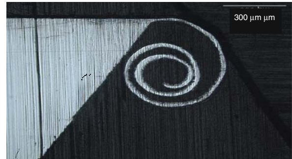
Fig. 7 Typical burr shapes in surface grinding and closeup of “Karpu” burr, [6]
