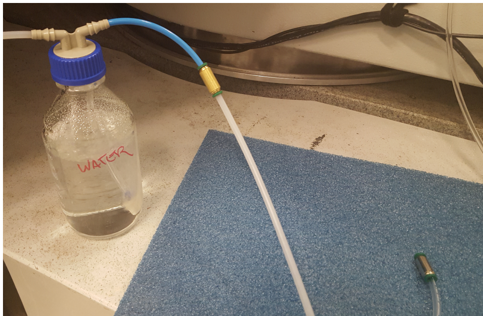
Figure 7.13: A distilled water bubbler was used for humidity control. This could be connected to the main N 2 flow control with the use of two valves. This allowed for on (high humidity) and off (low humidity) states.
