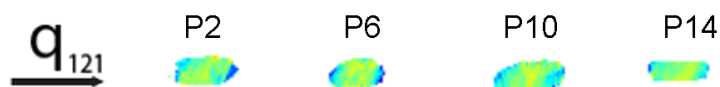
Figure 7.6: Multiple CsPbBr 3 crystals show strain at particle edges. Its consistency across scans suggests that it is not an artifact of the reconstruction, but a property of the crystal or substrate. The direction of the scattering vector \mathbf{q}_{121} is indicated. See Figure 7.1 to see the corresponding lattice plane. It is unclear what the source of the tensile strain is for these crystals. One possibility is that since the crystals are likely to agglomerate together in multiples of two or three (see Figures 7.2, 7.7, and 7.8), the strain is due to another physically touching or connected nanocrystal.
