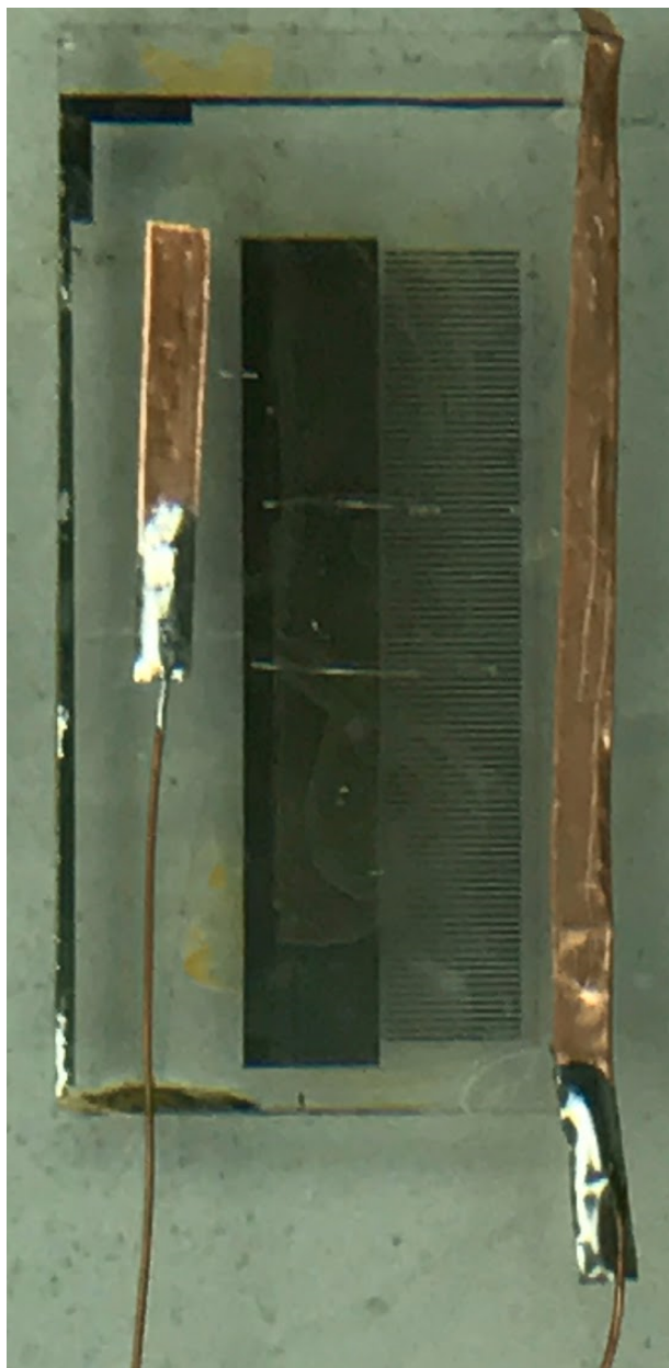
(a) A wire-bonded perovskite sample for XPCS. The wire bonds are visible as thin vertical strands near the center of the image. The Cu tape is stuck to the large part of each Au/Pt electrode, and wire is soldered onto the Cu tape. Wire bonds are connected between the finger electrodes and the larger pad, or the Cu tape itself if needed. The wires are soldered to a BNC connector which allows for a sealed sample chamber while applying a voltage across the sample.
