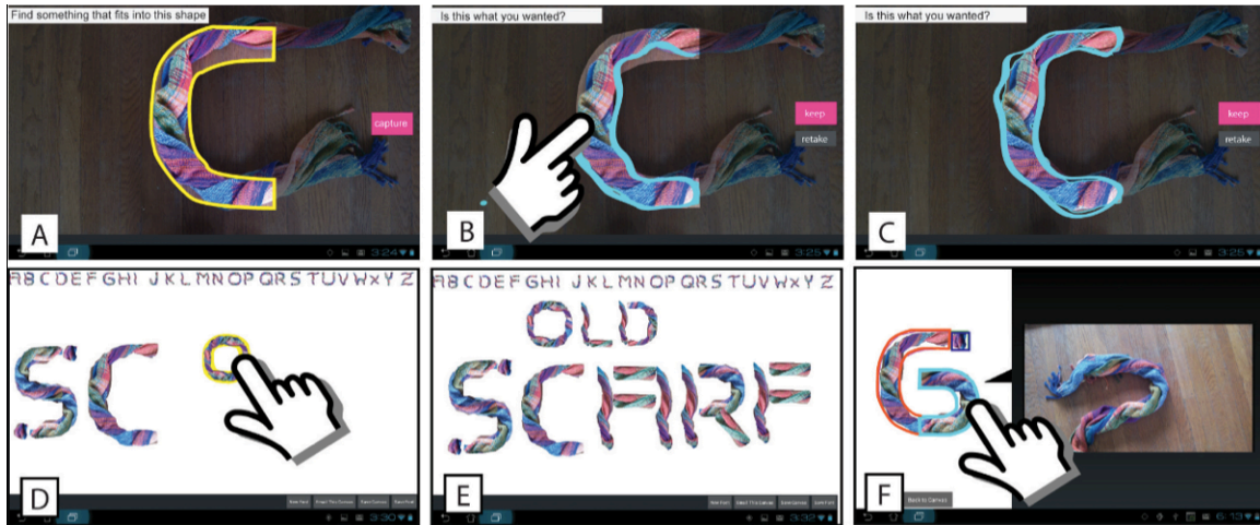
Figure 1: A) The user looks onto their environment through a shaped frame and captures (photographs) an object in this shaped frame. B&C) After capturing the shape, the user can edit by drawing a custom outline for the shape. D&E) After capturing all five shapes, the user is presented with their personal alphabet in the composition mode. The letters can be dragged, scaled and erased with fingers. F) In the history view, the user can see the original photographs that were used to compose each letterform
