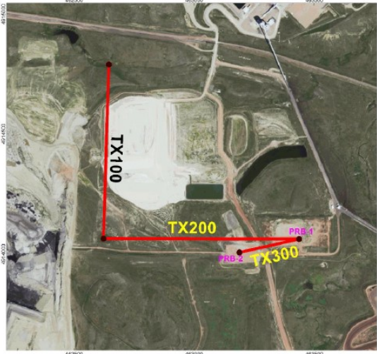
Figure 6. Enlarged view of the CSEM source locations used in the Wyoming CarbonSAFE EM measurement campaign.
