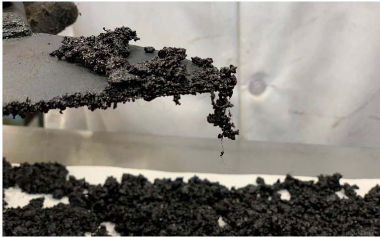
Figure 2.2: Asphalt mix reinforced with aramid fibers.
