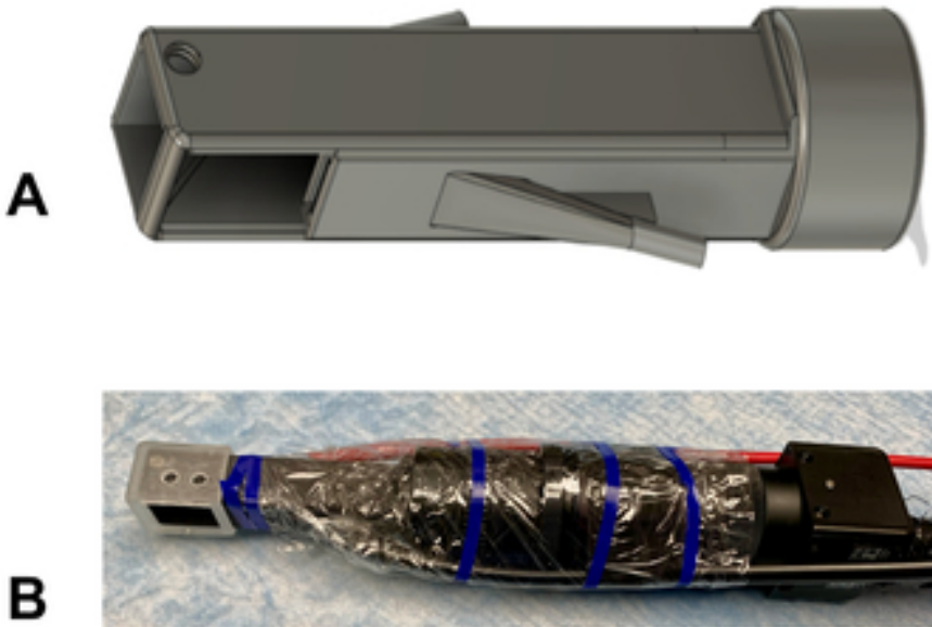
Figure 6.1 3D Printed SWIR Imaging Probe
