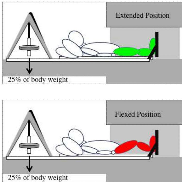
2. Loading device, custom made, for axial loading during MRI. Weights were hung behind the patient. Pulleys and the loading plate transmit the compressive force on the foot and load the knee joint.
