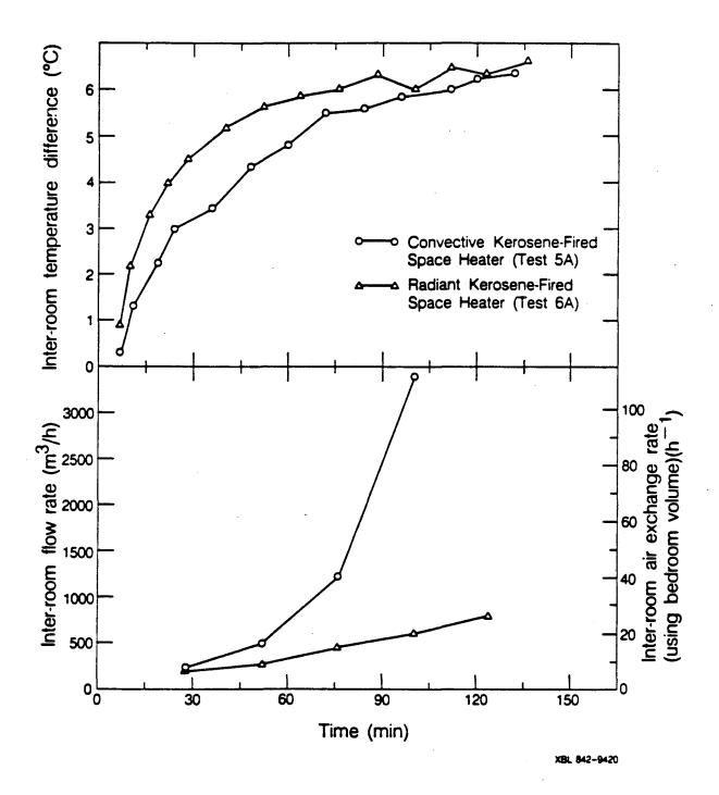
Figure 1. Inter-room temperature differences and air flow rates due to the use of a kerosene-fired space heater in a  $31-m^3$  bedroom. Flow rates were calculated using a two-compartment mass-balance model between the master bedroom and the rest of the house. The bedroom door was fully open during these tests.
