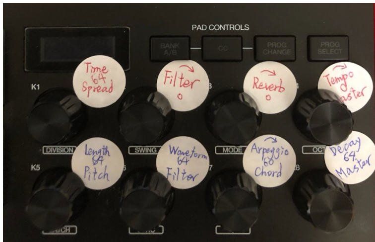
Figure 13. The mapping for the knobs in “Duet” and “Trio” pitch, while knob six adjusted wave position, filter frequency, and filter resonance. Knob seven activated the arpeggiator and major triad device, while knob eight controlled amplitude decay time and volume, as depicted in Figure 13.
