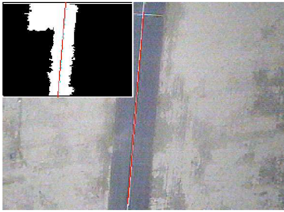
Fig. 3. Our previous experiment [27]. First vision-based UAV navigation on outdoor environment without artificial markings. The experiment was done on a short runway. The road detection was based on off-line learning (supervised) of lane marking and road pixel colors.
