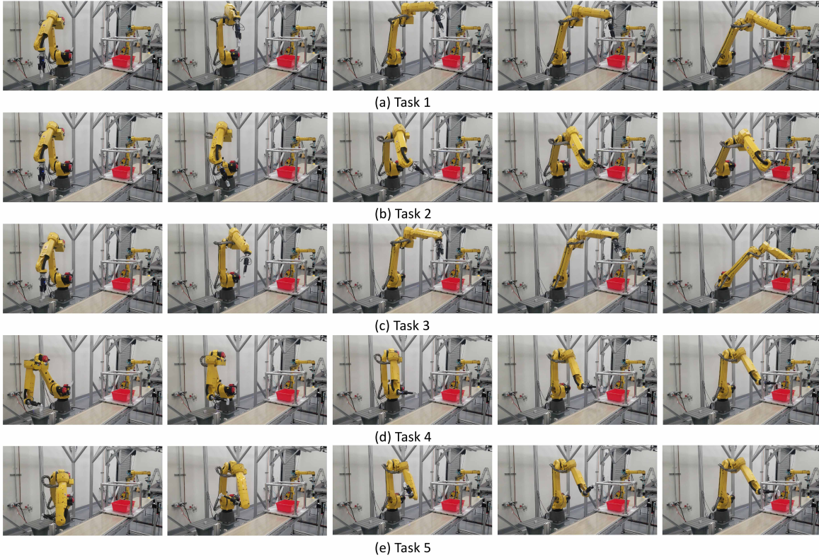
Figure 3.9: Sequences of snapshots of two different tasks. A FANUC robot is able to grasp a bottle and place it inside the cage with different final poses without collision.
