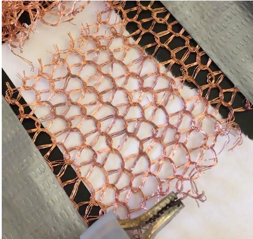
Figure 3.12. Suspected corrosion of copper mesh indicated by the darker spots. Note: pictured here is a troubleshooting setup and not the setup used for testing.
