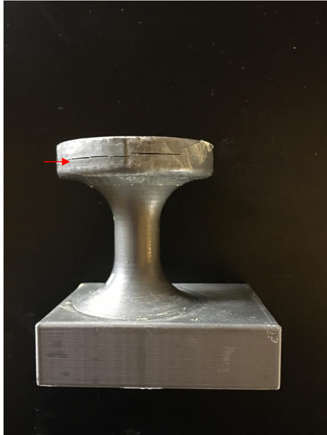
Figure 2.7. First version of the build plate extension made of PLA by an FDM 3D printer. The cracks (highlighted by the arrow) that led to uptake of resin can be seen near the top. It should be noted that the cracks were only hairline when the issue was discovered and have gotten worse from the removal of the glass disk and adhesive. Notice, too, that the shape varies from the second version. The first version was made to directly attach to the elevator rather than act as an augment of the existing build plate.
