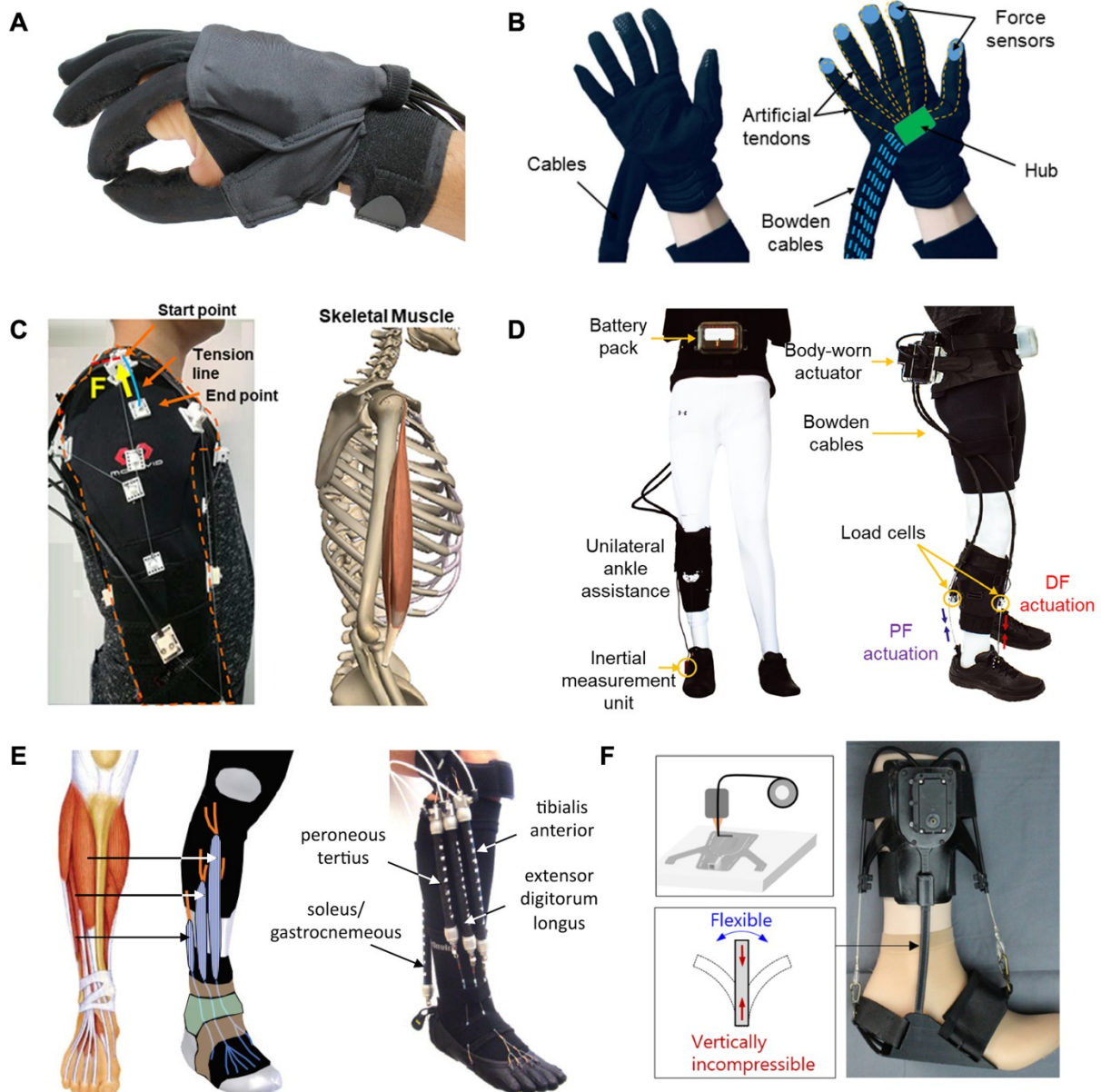
Figure 13. Soft actuators for disability rehabilitation. A) A pneumatic soft actuating glove for hand rehabilitation. Reproduced with permission. [394] Copyright 2016, IEEE. B) Motor glove with animation of tendon design for hand rehabilitation. Reproduced with permission. [158] Copyright 2021, IEEE. C) Bio-inspired soft exoskeleton for upper limb rehabilitation to reduce stroke-induced complications. Reproduced with permission. [493] Copyright 2021, IOP
