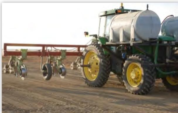
**Figure 10.** Close-up view of modified Orthman 1tRIPr strip-till row units at Sano Farms, showing the residue-cutting wheel and couler, subsoling shank, wavy coulters, and clod-busting rolling baskets.
