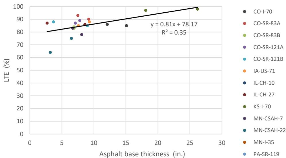
**Figure 4.5: Comparison between LTE measured with FWD and thickness of asphalt measured from cores.**
