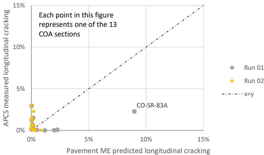
**Figure 4.2: Comparison between Run 02 predictions (50% reliability) and measured cracking (Run 02 overlay thickness is based on GPR).**
