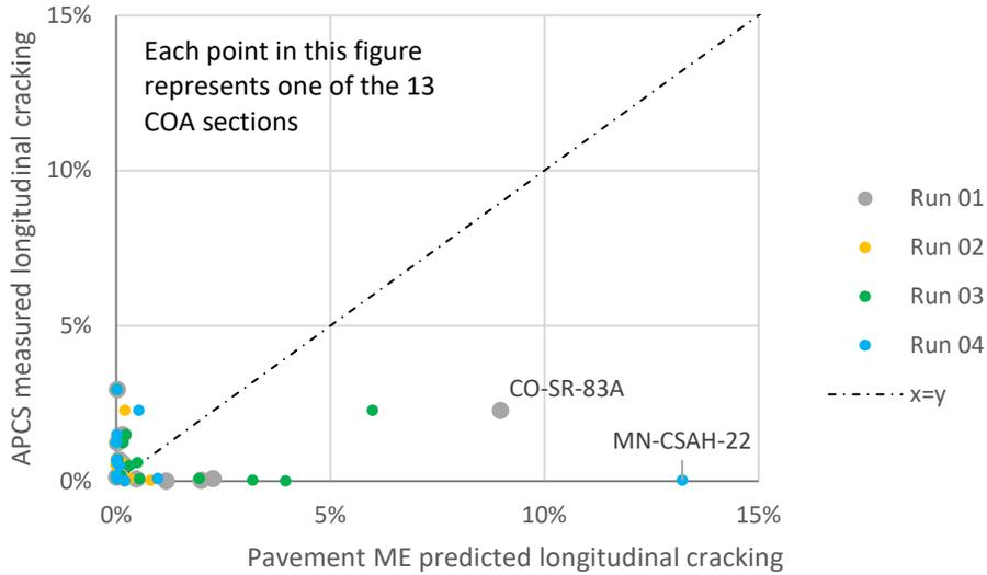
**Comparison between *Pavement ME* (50% reliability) and measured cracking.**
