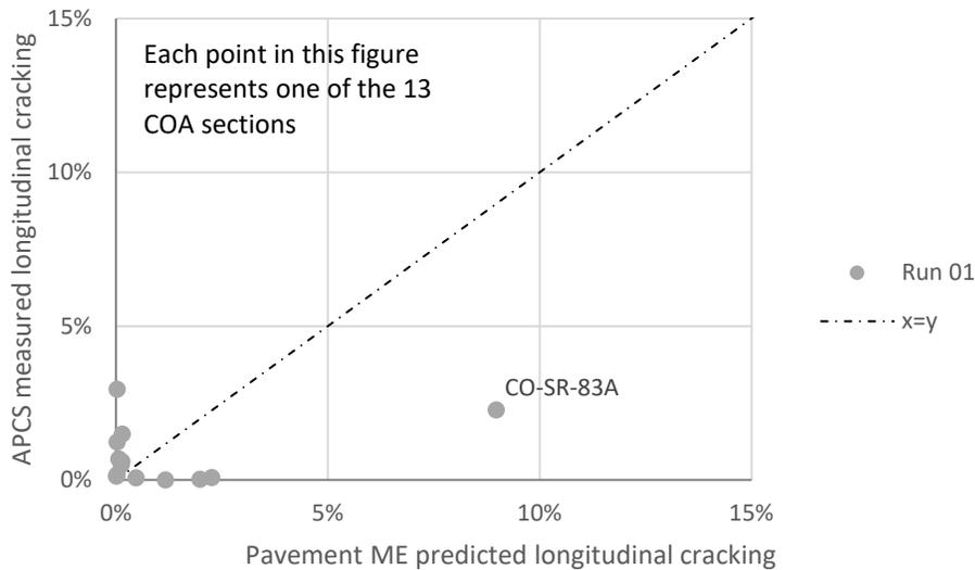
**Figure 4.1: Comparison between Run 01 predictions (50% reliability) and measured cracking.**
