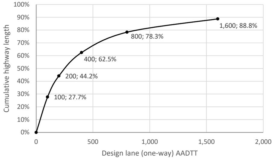
**Figure 2.1: Truck volume in Caltrans's non-interstate highway network.**
