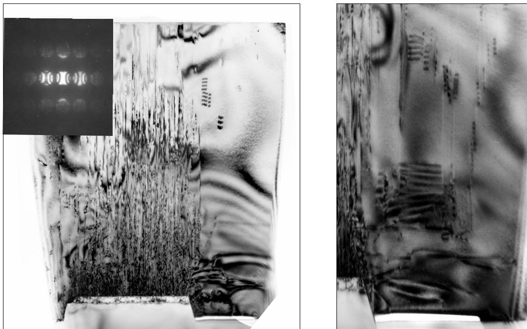
Fig. 5. TEM micrographs of cross-section uncoalesced pendeo-epitaxial layers grown on a-plane of 4H SiC. High density of defects (mainly stacking faults and dislocations) is observed in the seed area. An inset shows CBED pattern indicating that wider wing is growing with Ga polarity. Bending of dislocations occurs in this wing in the area close to the substrate. A gap between this wing and the substrate is formed for about 500 nm from the original seed and then it starts to touch the substrate. This is shown much clear in (b) which was taken from another wing (magnified). This also shows stacking faults on c-plane (SFc) and on prismatic planes (SFp).
