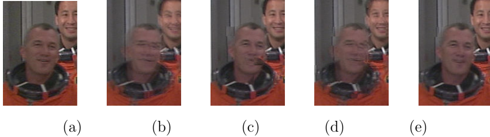
Figure 5.4: Zoom in for interpolated frame 185 in CREW (a) original frame, (b) bilinear interpolation, (c) 3D Recursive Search, (d) Phase Plane Correlation, (e) proposed method.
