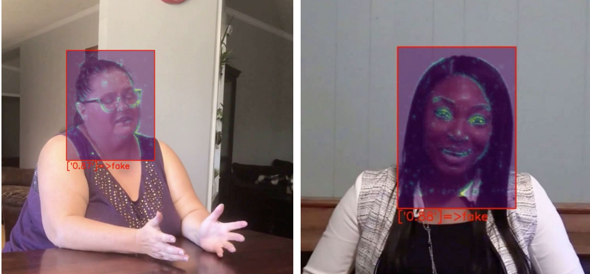
Figure 3.2. Gradient saliency maps obtained on Deepfake videos using guided backpropagation on a CNN-based detector [143]. The highlighted areas indicate the image regions that strongly influence the detector’s predictions.
