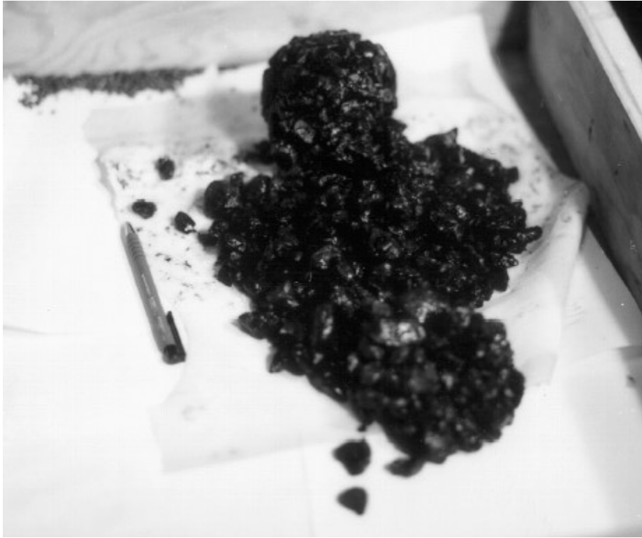
Figure 4.10. Goal 1 ATPB Specimen Failed in Saturated Permanent Deformation Test.
