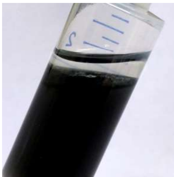
Figure 5. Extraction of product with MTBE from Black Water.
