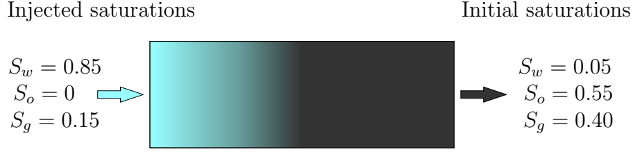
Figure 19. Sketch of the water-gas injection problem. Water and gas are injected into a medium initially filled with oil and gas.
