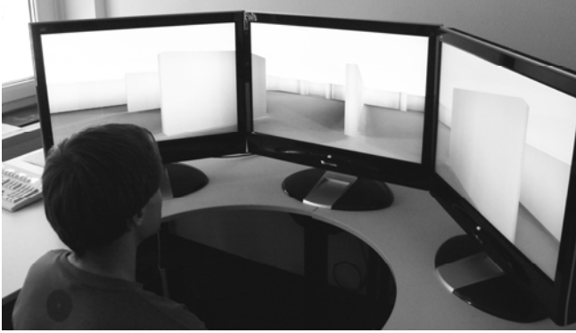
Figure 1: Setup of the immersive virtual environment with three screens. The horizontal field of view of about 170° allows peripheral vision.
