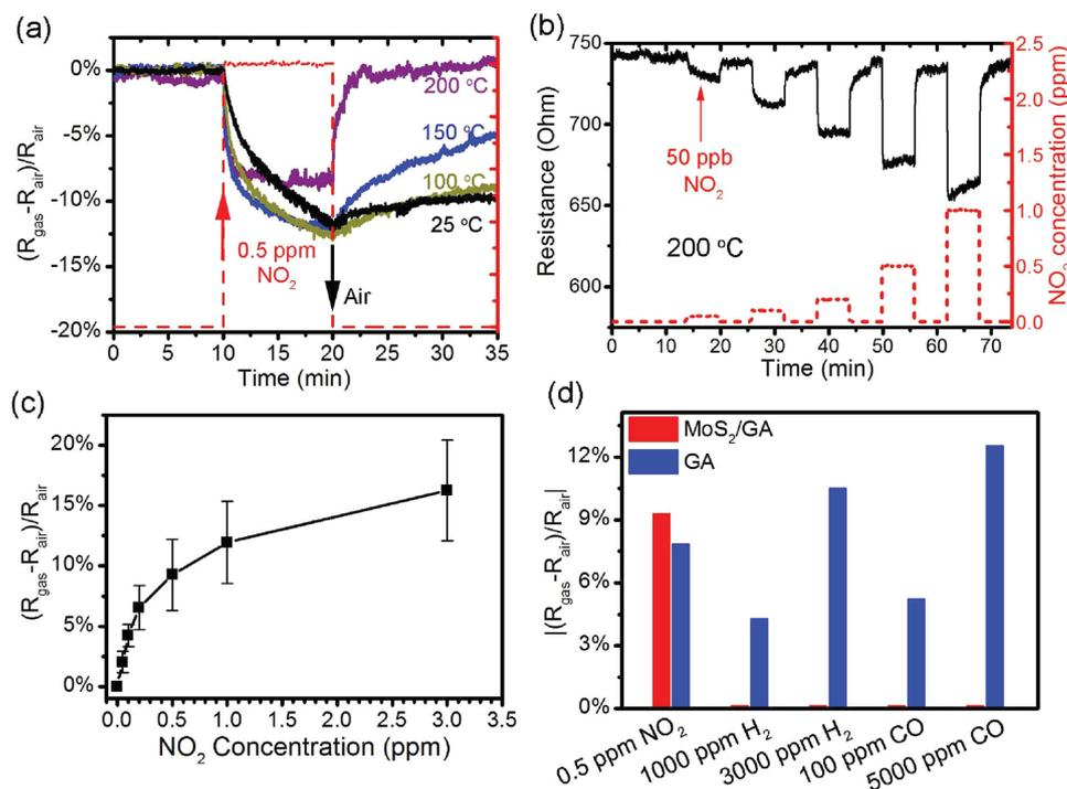
**Figure 5.** a) Sensor response to 0.5 ppm NO<sub>2</sub> at various microheater temperatures, displaying improvement in response and recovery time. b) Real-time resistance change of the sensor with the microheater temperature of 200 °C. c) Response versus NO<sub>2</sub> concentration for microheater temperature of 200 °C. d) Selectivity of the MoS<sub>2</sub>/GA sensor compared to GA alone for microheater temperature of 200 °C.
