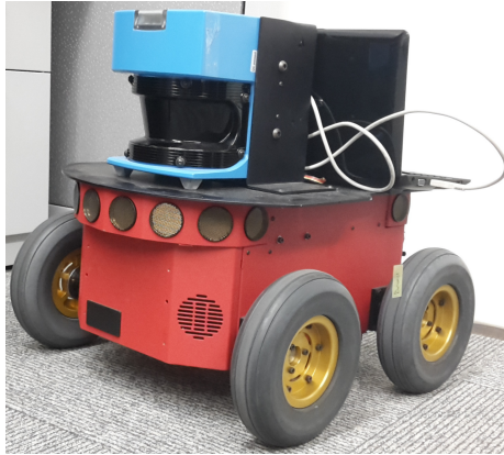
Figure 4.21: The P3AT robot used to test the HCMDP planner in the real world.
