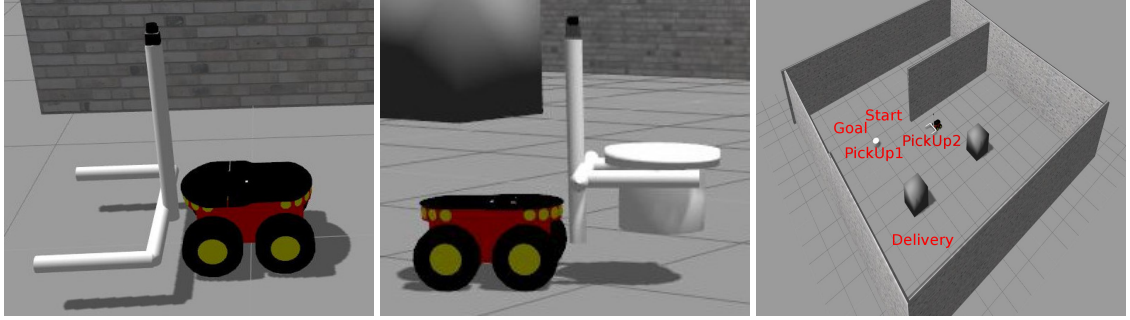
Figure 5.6: On leftmost figure, the autonomous vehicle with its gripper fully opened at its lowest position. In the center figure, the vehicle carrying an object. Note that the fork as been closed and lifted. On the right, the environment used for testing.
