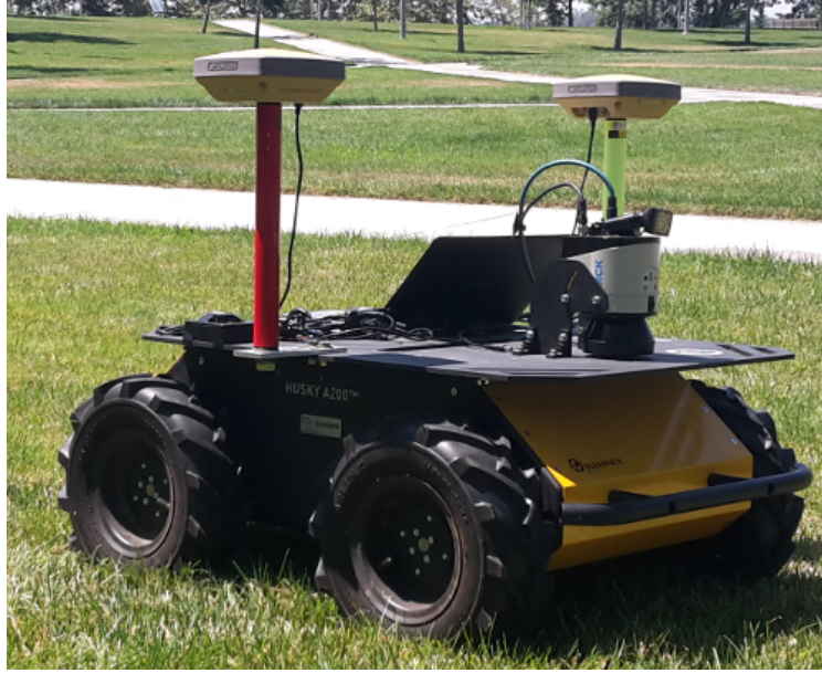
Figure 5.14: The Husky robot used to validate the planner proposed in the paper.
