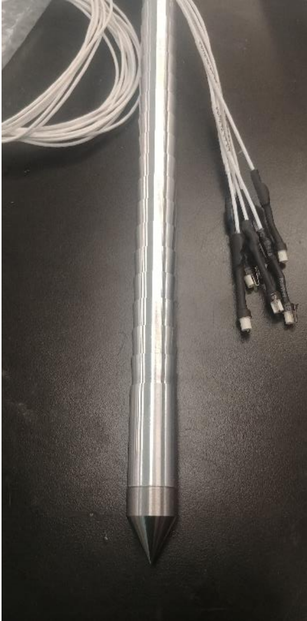
Figure 1.3. Internally instrumented pile with shaft geometry modelled after snake ventral scales.
