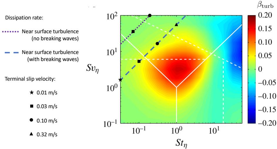
**Figure 3.** Isocontours of  $\beta_{\text{turb}} = (w_{t,\text{eff}} - w_t)/W$  on the  $St_\eta$ - $Sv_\eta$  plane obtained from DNS of homogeneous isotropic turbulence at  $Re_\lambda = 140$ . Here  $W$  is a turbulence velocity scale. Figure adapted from Good et al. (2014).
