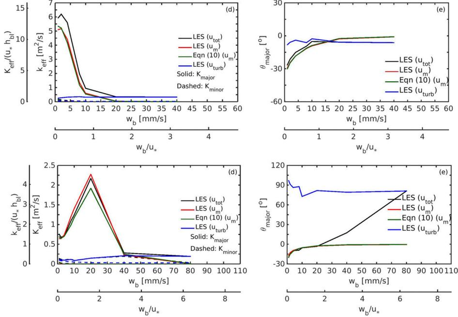
**Figure 15.** Equivalent horizontal diffusivity and axis of rotation for OML driven by wind shear (upper panels) and in Langmuir turbulence (lower panels) as a function of floatability parameter (here denoted as  $w_b/u_*$ ) for buoyant material. Reproduced from Liang et al. (2018).
