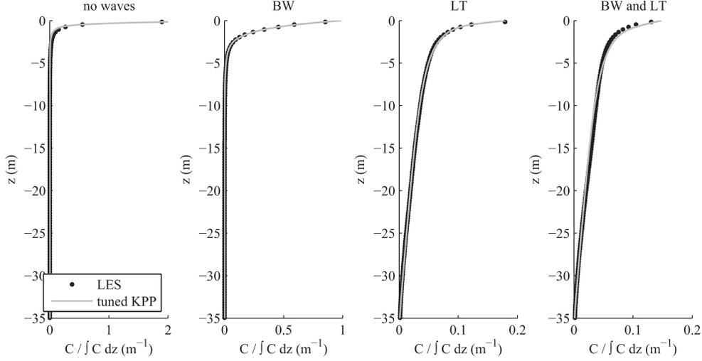
**Figure 12.** Normalized vertical profiles of mean concentration obtained from LES (symbols) and from the analytical model given by Eq. (43) using the parameterizations given by Eqs. (37) and (44) for an OML driven by (from left to right) (i) wind shear, (ii) wind shear and breaking waves, (iii) wind shear and Stokes drift, and (iv) wind shear, breaking waves, and Stokes drift. Figure reproduced from Kukulka and Brunner (2015).
