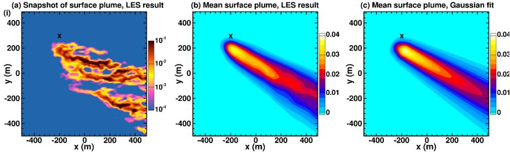
**Figure 10.** Surface concentration for particles with  $Db = 3.2$  in Langmuir turbulence: (a) instantaneous plume, (b) time-averaged plume, and (c) Gaussian fit to the time-averaged plume. Black cross symbol indicates the horizontal location of the underwater source. Reproduced from Yang et al. (2015).
