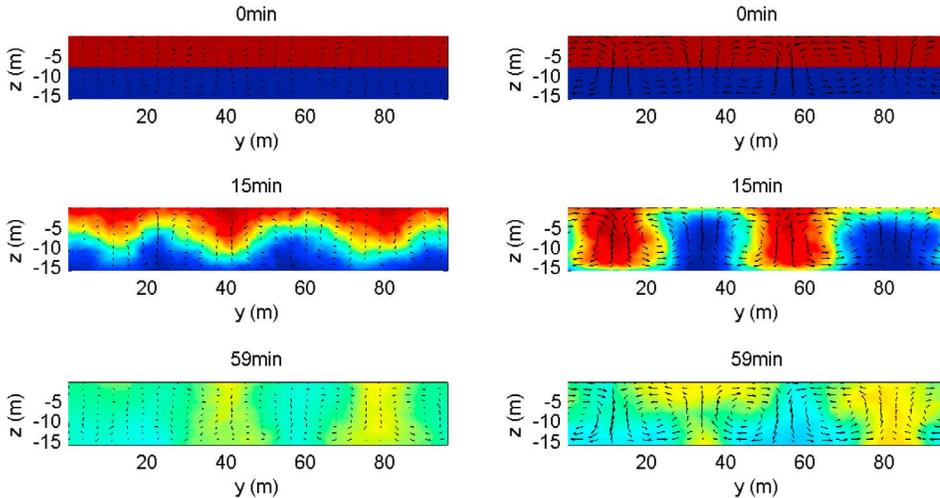
**Figure 7.** Time evolution of tracer concentration field (averaged in the cross-wind direction) for coastal ocean driven by wind shear (left panels) and Langmuir turbulence (right panels). Note that after 15 min the tracer is well mixed in the vertical direction for the Langmuir turbulence case, but the horizontal patchiness persists even after 59 min. Reproduced from Kukulka, Plueddemann, and Sullivan (2012).
