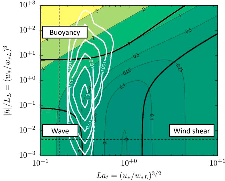
**Figure 5.** Regime diagram for turbulence in the OML. Colored contours show the logarithm of the normalized TKE dissipation rate  $\log_{10}(\epsilon|h|/u_*^3)$ . Thick solid lines divide the regime diagram into regions dominated by one forcing (buoyancy-driven, wind shear-driven, and wave-driven OML). White contours show the joint PDF of  $La_t$  and  $|h|/L_L$  for the Southern Ocean winter. Figure adapted from original by Belcher et al. (2012).
