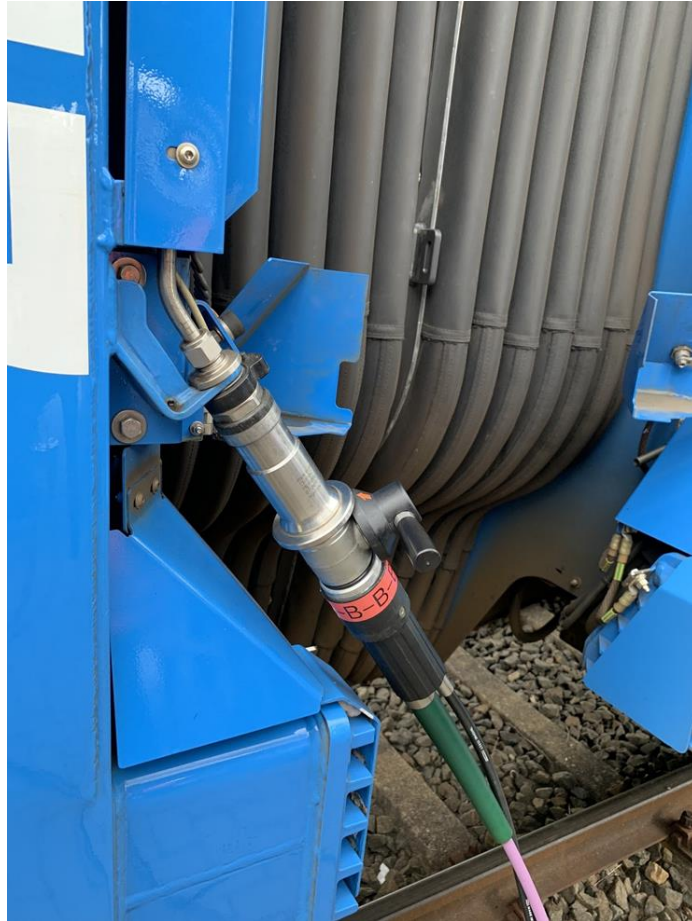
Figure 58: Refueling a Multiple Unit Vehicle with Hydrogen
