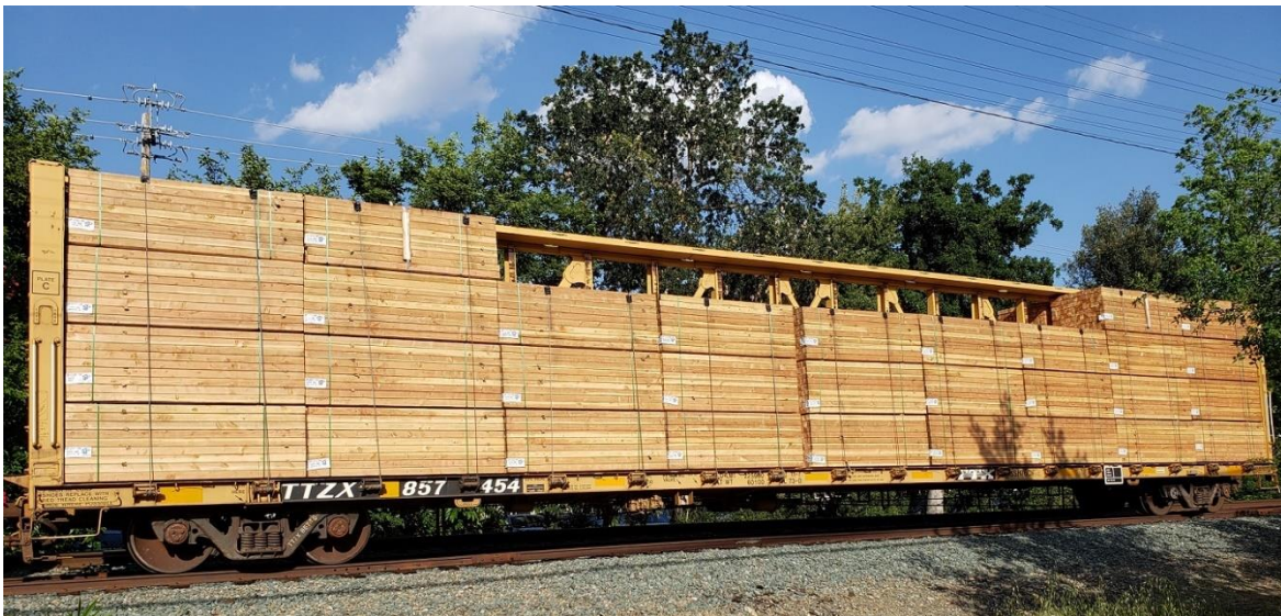
Figure 16: Wood Being Carried on a Centerbeam Car, Davis, CA May, 2019 (Photo from author's collection) This configuration is one of the car-commodity combinations that was modeled.
