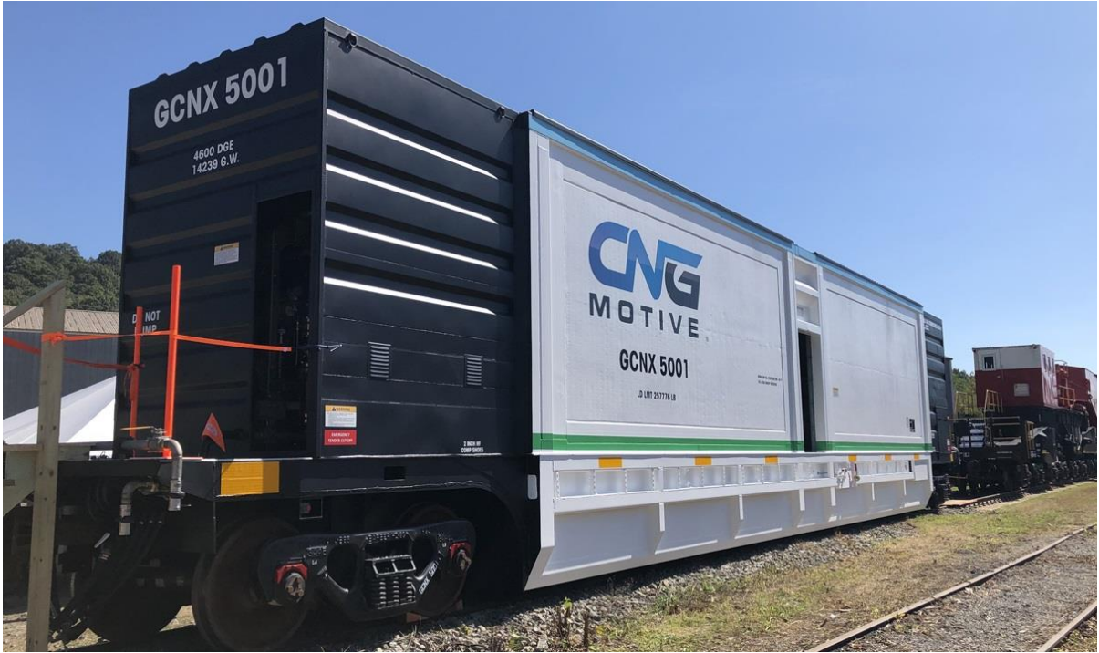
Figure 4: A CNG Tender Recently Developed by CNGmotive Photo courtesy of William C. Vantuono, and Railway Age (with permission granted)
