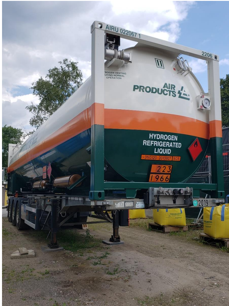
Figure 5: A Thermally, Vacuum-insulated, Stainless Steel Tank from Air Products (Photo from author's collection)
