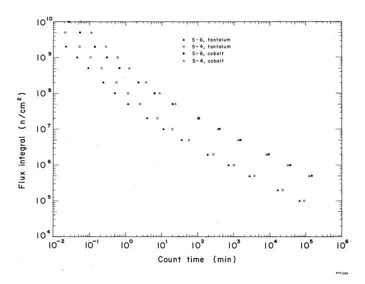
Fig. 3. Comparison of performance of S-4 and S-6 spectrometer systems for counting  ${\rm Co}^{60}$  and  ${\rm Ta}^{182}$  in small disk samples.
