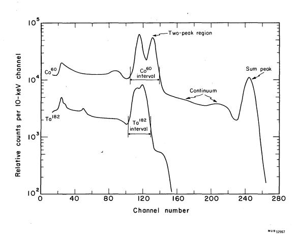
Fig. 1. NaI(Tl) scintillation crystal gamma-ray spectra of  ${\rm Co}^{60}$  and  ${\rm Ta}^{182}$  observed in activated disks.
