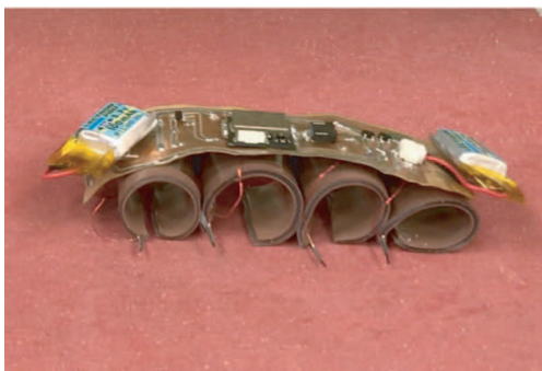
Fig. 7.2 (a) Caterpillar-inspired robot made out of 4 actuator segments connected in series, with embedded flexible circuit and battery packs on top. (b) Tethered starfish-inspired robot made out of 7 actuator segments that produces a rolling motion when activated. Both pictures are courtesy of the Soft Machines Laboratory at Carnegie Mellon University.
