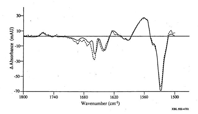
Figure 6.12 Discrete least-squares approximation of the 260 K, M - bR spectrum of glucose-embedded specimens to Ormos' first 260 K difference spectrum. The two spectra are superimposed with the glucose-embedded PM spectrum as a solid trace, and Ormos' difference spectrum as a dashed trace.
