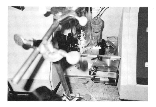
wires are seen exiting from the top of the picture. Two wires are led through an orifice in the cryostat and make contact with the brass specimen holder.
