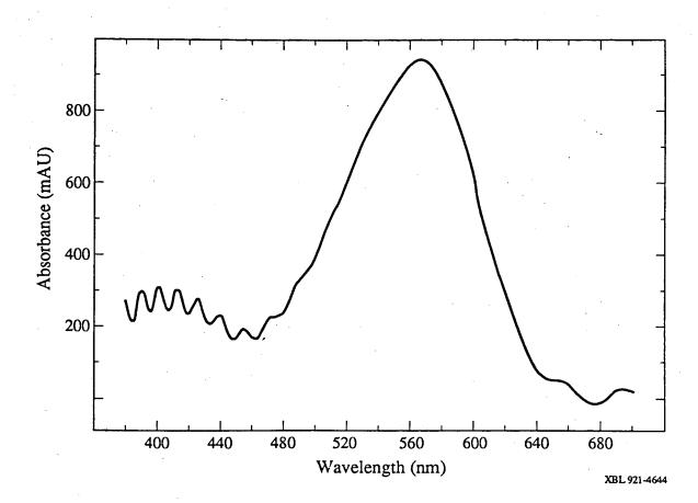
spectrum. The Aminco sits on a lab bench and while the scan was running, I did not touch it. I discovered, though, that seating myself or walking around caused these spikes. As a test, I stood in place during the scan except when the spectrophotometer was scanning between 540 and 585 nm. Figure 2.5 shows the results. The trace is smooth except during the portion of the scan when there was movement in the room. For subsequent scans, I limited my movement; the problem was alleviated.
