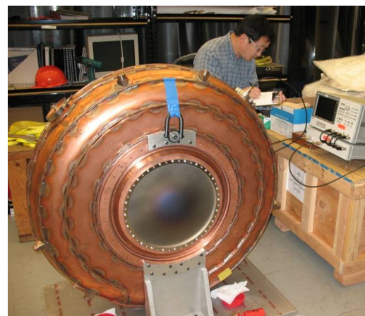
Figure 5: MICE RF cavity measurements with curved beryllium windows at LBNL.
