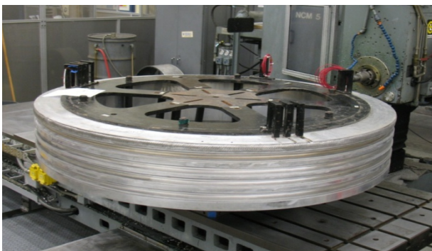
Figure 3: Cold-mass received from China, and currently at LBNL for welding of the LHe pipes and preparations for testing at Fermilab.
