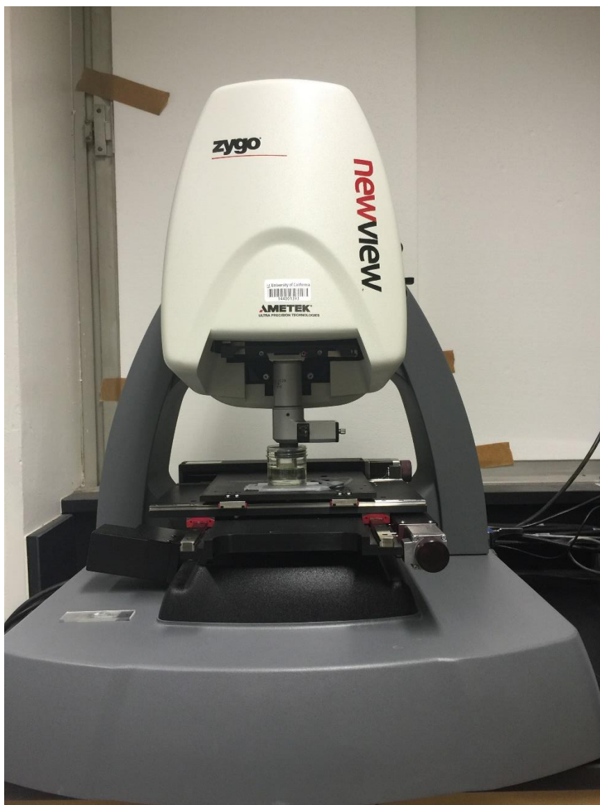
Figure 8.5 Photo of VSI instrument (NewView 8200, Zygo Corporation)
