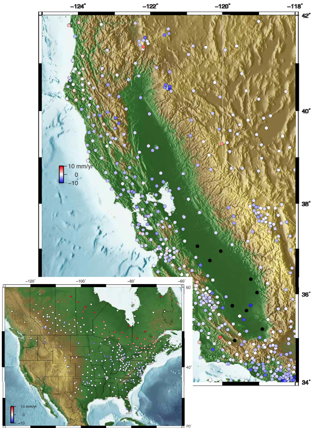
Figure 12. Vertical Displacement Rates from Continuous GPS Stations in North America. Inset, vertical rates from Sella et al. (2007). Main frame, vertical rates from the most-recent PBO solution ( http://pboweb.unavco.org/ ).
