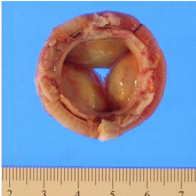
Figure 4B: Photograph of explanted stenotic mitral valve bioprosthesis (originally a 27 mm bovine mitral valve bioprosthesis), atrial view
