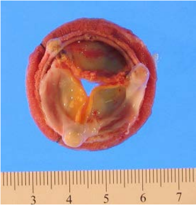
Figure 4A: Photograph of explanted stenotic mitral valve bioprosthesis (originally a 27 mm bovine mitral valve bioprosthesis), ventricular view
