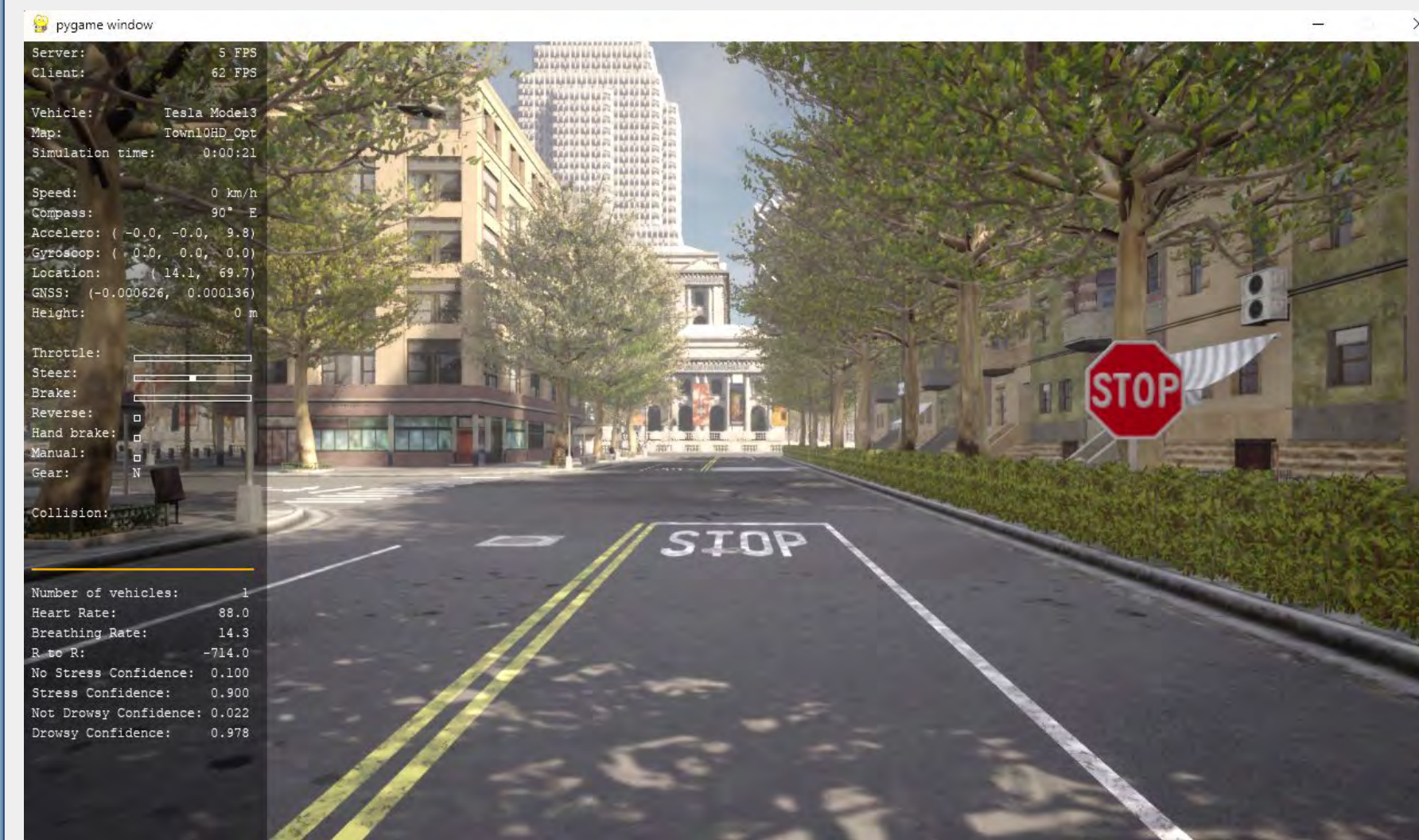
Fig. 2: CARLA displaying driver's biometrics, vehicle controls and model confidence values.
